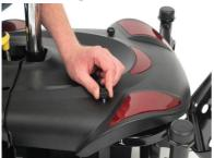
2. Connect the battery pack. Refit the front shroud and tighten the two knobs to secure.
