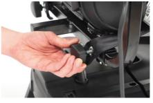
6. Plug the cable from the joystick remote in to the port at the back of the powerchair base.
