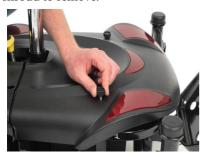
4. Disconnect the batteries and lift up the battery pack to remove.
