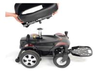
3. Loosen and remove the two knobs on the shroud. Lift up the front shroud to remove.
