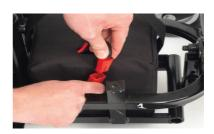
5. Lift up the yellow handle to separate the chassis. This can be done with or without the batteries installed.
